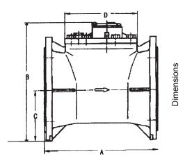
NOTE: Flanges are ANSI Class 150 raised face flanges. Bolt Pattern: 2" & 3" - 4 holes, 4" & 6" - 8 holes.
